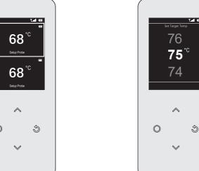
Tap the confirm button to open the target temperature setting screen. Tap the forwards and backwards buttons to select the target temperature.
